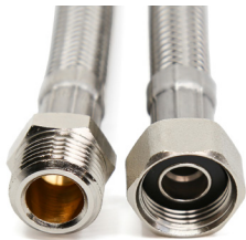
Example of suitable flexible hose connections: G 3/8" swivel nut for connection to the UVC-LED module and G 3/8" male thread for connection to the water installation.
